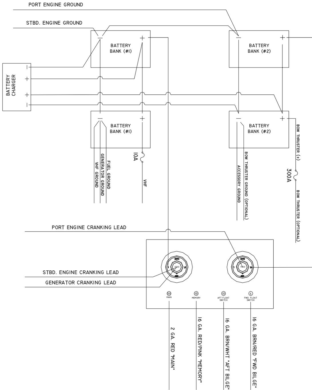
TYPICAL OUTBOARD SWITCH PANEL WIRING
