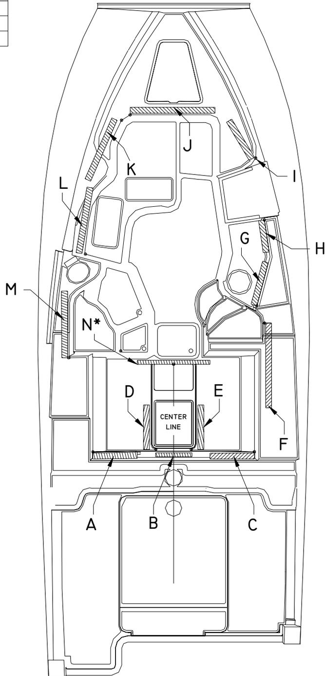
ACCESS PLATE AND RIGGING TUBE LOCATIONS
